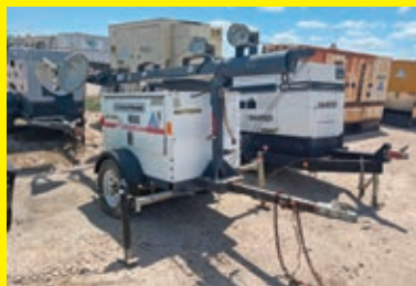
LOT 119: MAGNUM PRO MLT3060M LIGHT PLANT SN:1401795 powered by diesel engine, equipped with 4-1,000 watt lightbulbs, 6KW, trailer mounted.
