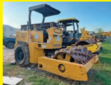
LOT 143: CAT CP433B VIBRATORY ROLLER SN:1MG00514 powered by Cat diesel engine, equipped with OROPS, 66in. padfoot drum, vibratory drum, drum drive.
