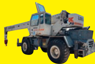
LOT 131: KOEHRING LRT275D ROUGH TERRAIN CRANE SN:79962 powered by diesel engine, equipped with Cab, 27.5 ton capacity, 72ft. reach.
