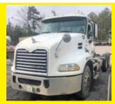
2014 MACK CXU613 VN:40445 powered by Mack MP7-395C diesel engine, equipped with M-drive automatic transmission, power steering, 2-line wet system, air ride suspension, polished aluminum front wheels, tandem axle. Missing 4-rear wheels, automatic control missing, Does Not Run.
