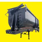
2015 MANAC 4L240A900 VN:154412 equipped with steel dump body, 85,000lb GVWR, barn door tailgate, spring suspension, steel wheels, 11R24.5 & 455/55R22.5 super single tires, tandem axle. Missing 2-11R24.5 tires, missing hoist cylinder, roll over damage.
