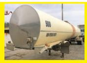
2005 POLAR SRJ3 VN:27995 equipped with 6500 gallon tank body, 68,000lb GVWR, tool box, air ride, 295/75R22.5 tires, tandem axle.
