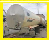
**2005 POLAR SRJ3** VN:27985 equipped with 6500 gallon tank body, 68,000lb GVWR, tool box, air ride, 295/75R22.5 tires, tandem axle.
