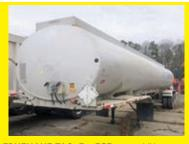
1991 FRUEHAUF TAG-F2-ESF-9200 VN:9307 equipped with 9200 gallon tank body, 4-compartments, hose tray, Flotech FT208 overfill monitor, 65,000lb GVWR, spring suspension, polished aluminum wheels, 295/75R22.5 tires, tandem axle.
