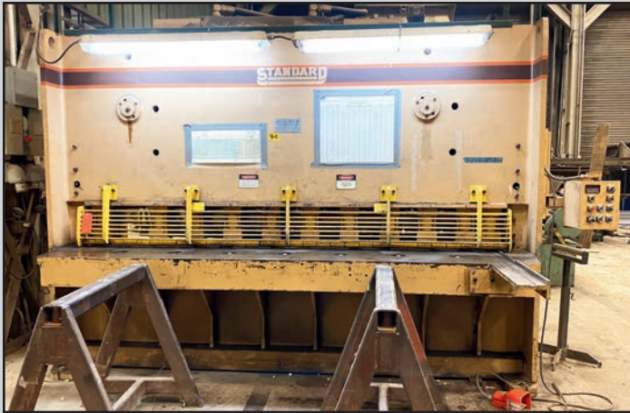
STANDARD INDUSTRIAL CORP. 10' x 3/4" HYDRAULIC PLATE SHEAR
