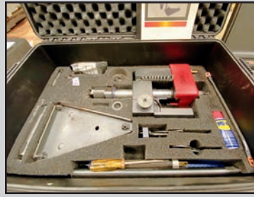
BORETECH 306-Z BORE WELDING SYSTEM WITH WIRE FEED AND CONTROLLER
