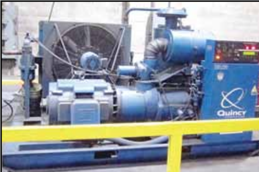
QUINCY QSI-750 150 HP AIR COMPRESSOR
